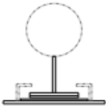
PIPE SLIDE & SLIDE PLATE TYPE - 35
